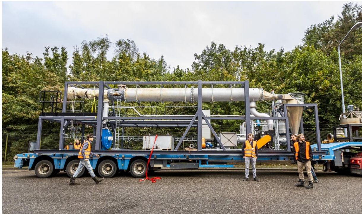
First industrial combustion pilot at Swinkels Brewery 100 kW
